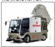
The total volume is approximately 3,5 m³, a capacity which reduces the down time required for emptying and therefore also the total cleaning time. It is vertically divided in two parts the lower part is designed for collection of material while the upper part houses the filter. The waste hopper is emptied by lifting it on vertical guides up to 1.800 mm.
