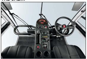
The cabin is comfortable because it is spacious and insulated with anti-vibration supports. It is comfortable to drive and the large windscreen provides maximum external visibility for the operator, making manoeuvring and control over collection are easier. The activation commands, simple and intuitive are grouped on a central console. The others are on the front part of the roof, both easily accessible from the working position. On request the machine can be
