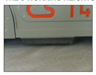
Comac has produced a special device to control vehicle height from ground which, acting separately on the four wheels, maintains constant the height from the ground, optimizing work and stability. This device can also maintain the height of the vehicle unchanged even when the load varies. The operator can position the machine on three different pre-established levels in order to meet various needs:
