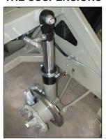
The four independent suspensions, whose regulation and control is assigned to an electronic control unit, are hydraulic with McPherson system on all four-wheels.
