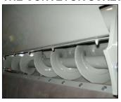
The screw conveyors consist of two steel shafts, both equipped with a spiral which, hydraulically moved, rotate on the same axis, conveying dirt and debris of different dimensions close to the suction outlet.
