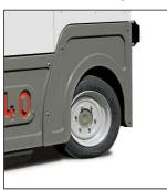
CS140 "TwinAction" has an integral steering system on all 4 wheels with symmetrical front and rear angles (the same centre of rotation for the two axles) and turning circle of 4,25 m. Together with great manoeuvrability, even near walls or fences, and guarantee the necessary ease of handling to operate in places where the space is limited such as historical town centres or cluttered areas, at the same time guaranteeing maximum vehicle stability during transfer even at the highest speed.
