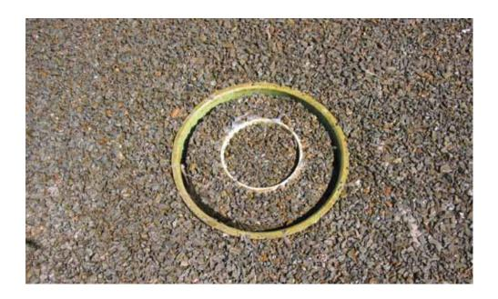
Both methods will provide a good indication of the condition of the surfaces. In general, most new surfaces have an infiltration rate that exceeds the requirement for a one hundred year storm. Therefore, absolute accuracy may be more than is needed to establish the need to restore a surface.
