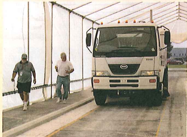
Pickup performance testing of an Elgin Crosswind regenerative air sweeper
