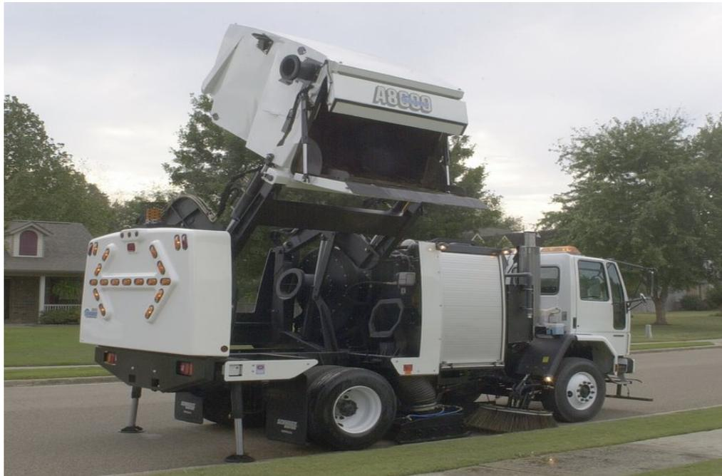
**Figure 9. Photographs of the Schwarze A8000 regenerative air sweeper used for the Seattle Street Sweeping Study.**
